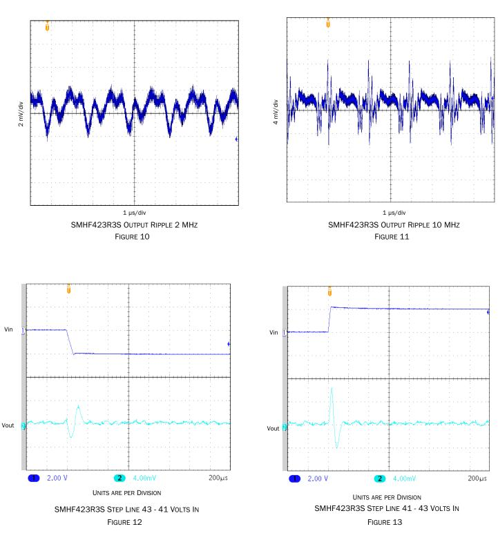
Typical Performance Plots: 25 °C case,  $42 V_{IN}$ , 100% load, unless otherwise specified. For reference only. Not guaranteed specifications.
