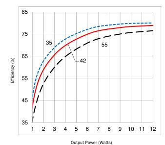
Typical Performance Plots:  $25 \,^{\circ}$ C case,  $42 \, V_{IN}$ , 100% load, unless otherwise specified. For reference only. Not guaranteed specifications.
