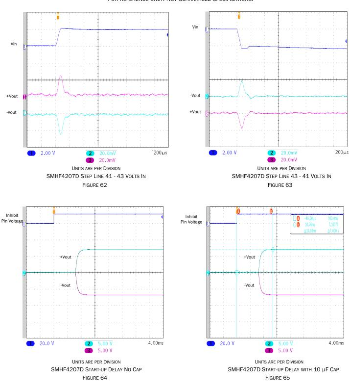
Typical Performance Plots: 25 °C case, 42 V<sub>IN</sub>, 100% load, unless otherwise specified. For reference only. Not guaranteed specifications.
