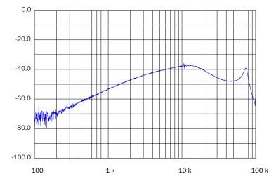
Frequency (Hz), 42 V<sub>IN</sub> SMHF4205S AUDIO REJECTION FIGURE 19
