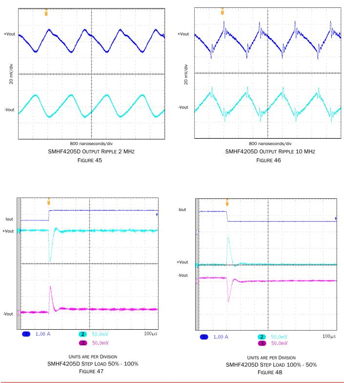
Typical Performance Plots:  $25^{\circ}$ C case,  $42 V_{IN}$ , 100% load, unless otherwise specified. For reference only. Not guaranteed specifications.
