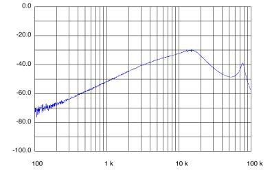
Frequency (Hz), 42 V<sub>IN</sub> SMHF4207D AUDIO REJECTION FIGURE 55
