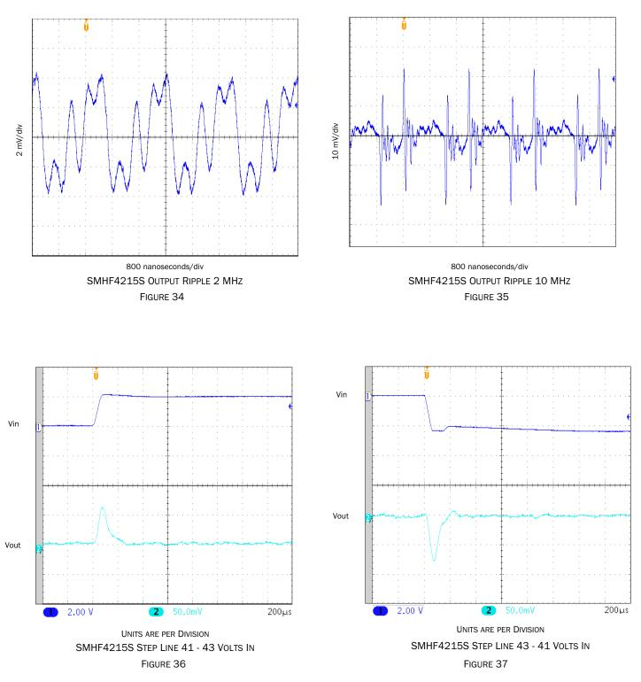
Typical Performance Plots:  $25^{\circ}$ C case,  $42 V_{IN}$ , 100% load, unless otherwise specified. For reference only. Not guaranteed specifications.
